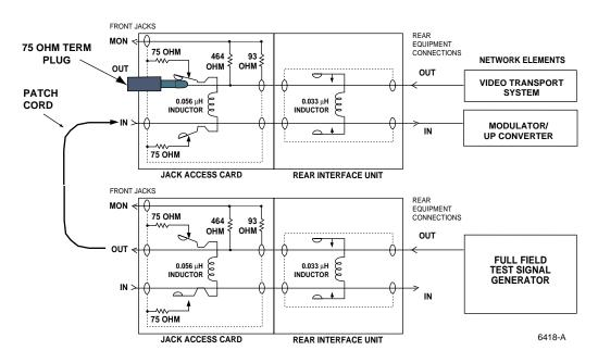
Figure 22. Intrusive Insertion of Test Signal
